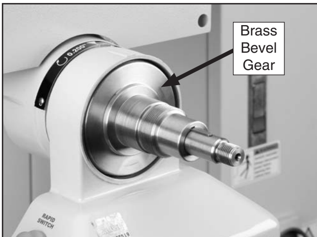
Figure 4. Brass bevel gear installed onto the leadscrew.
