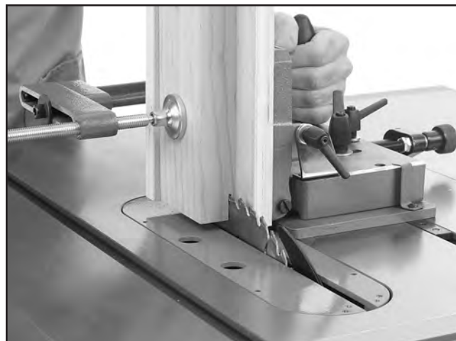
Figure 24. Making the first cheek cut.
