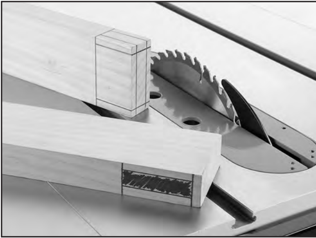
Figure 19. Mortise and tenon cutting lines.
