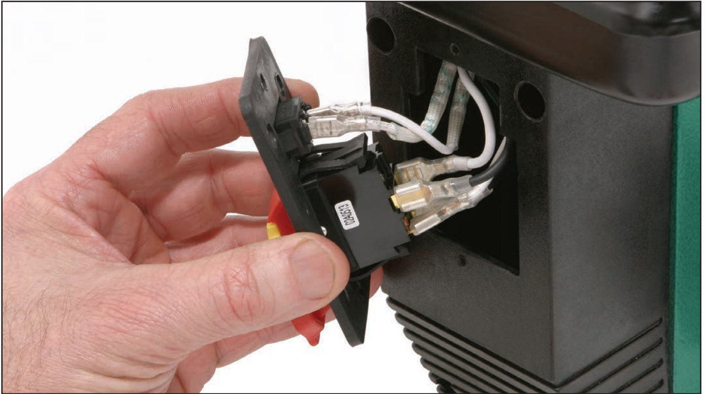
Figure 32. G9969 Switch Wiring.
