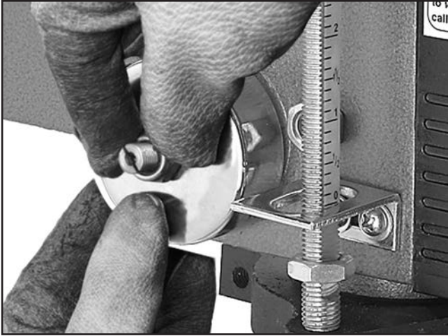
Figure 31. Loosening cover and jam nut.
