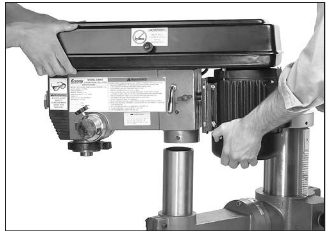
Figure 10. Mounting the headstock.
