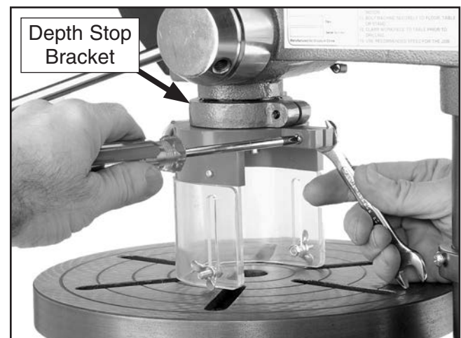
Figure 1. Example photo of installing chuck guard assembly.
