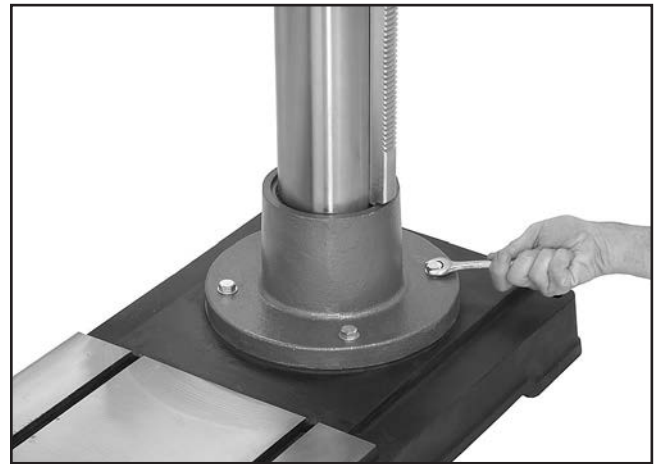
Figure 6. Assembled column and base.
