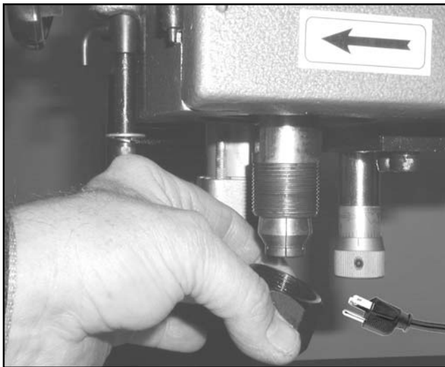
Figure 7. Installing collet nut.
