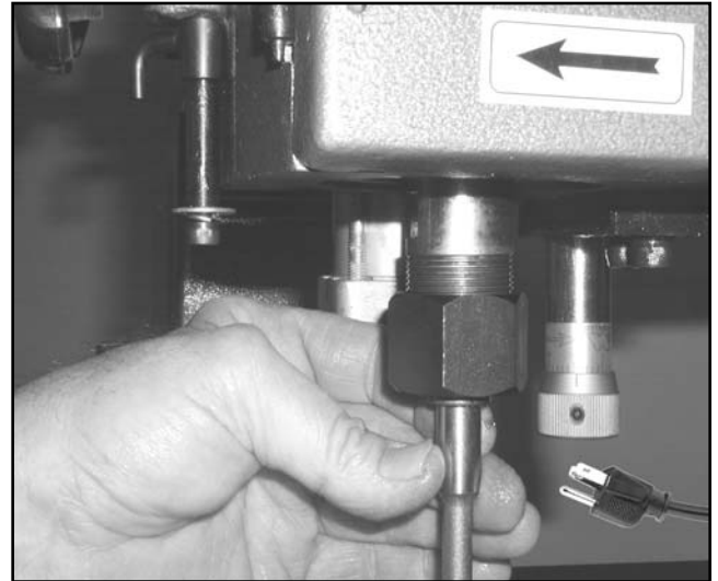
Figure 8. Installing the router bit.
