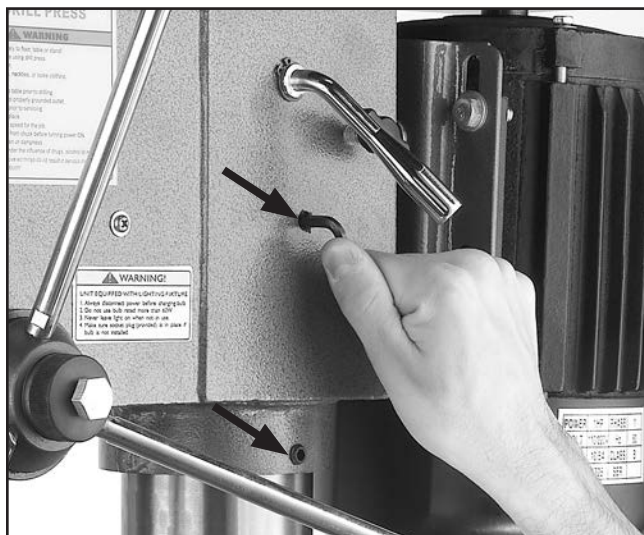
Figure 22. Securing headstock to column.
