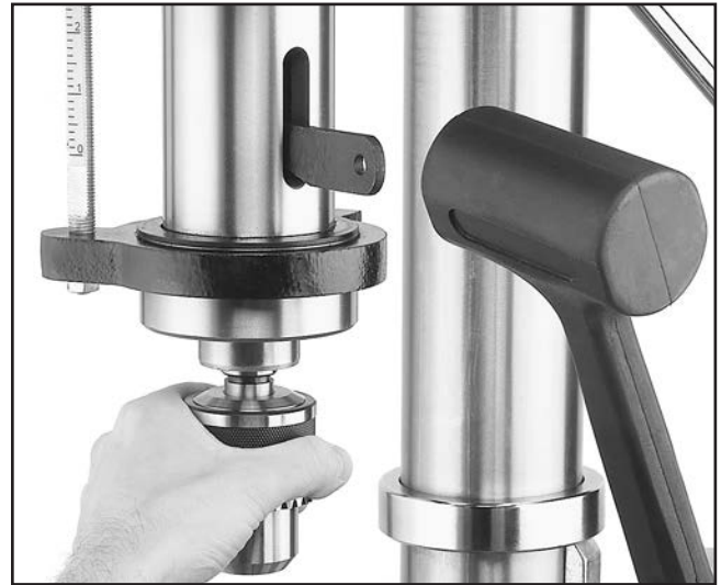
Figure 36. Using drift key to remove arbor.
