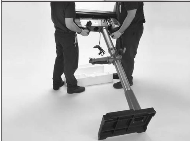
Figure 20. Tilting drill press upright.
