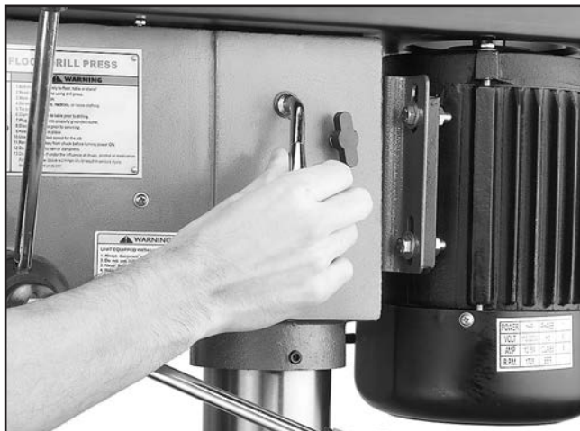
Figure 31. Using the belt tension lever.
