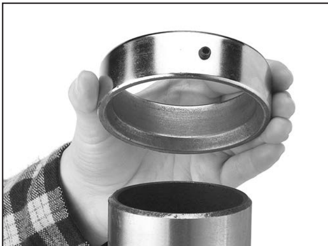
Figure 18. Correct column ring orientation.
