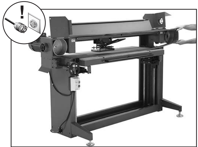
Figure 36. Installing new belt.
