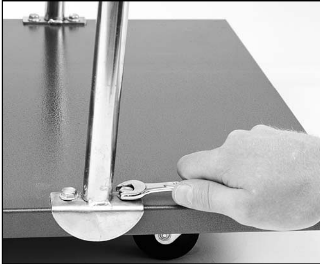
Figure 6. Mounting brackets to base.
