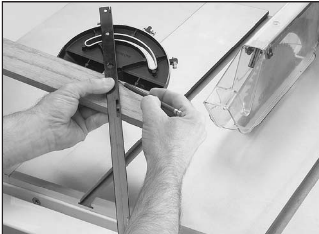
Figure 44. Marking miter line.
