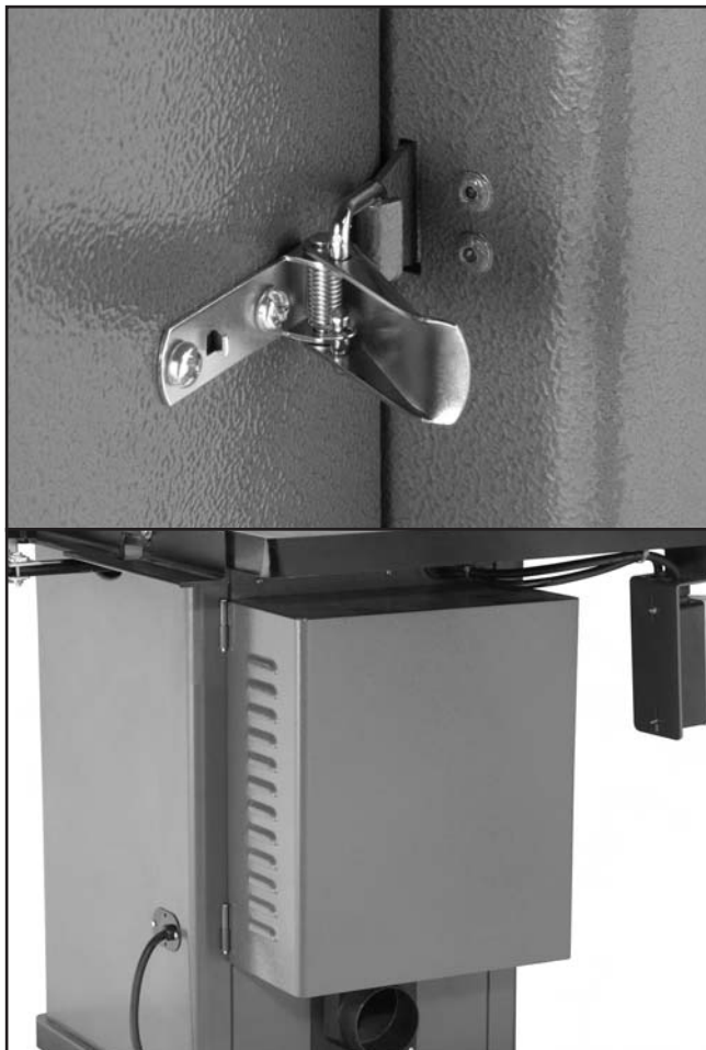
Figure 22. Motor cover installed on stand.
