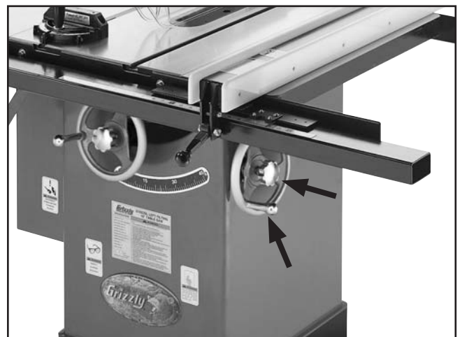
Figure 24. Handle and lock knob installed on handwheel.
