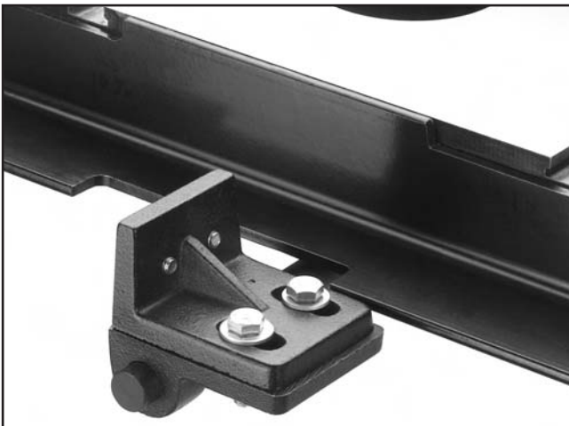
Figure 27. Splitter bracket installed.
