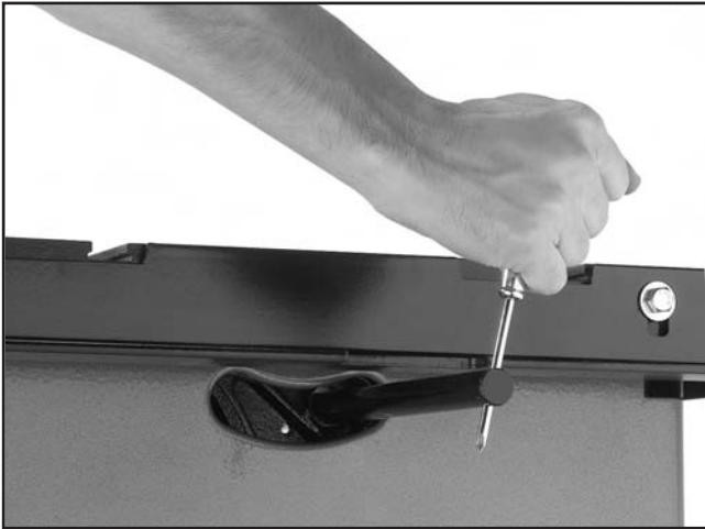
Figure 26. Attaching guard support shaft.
