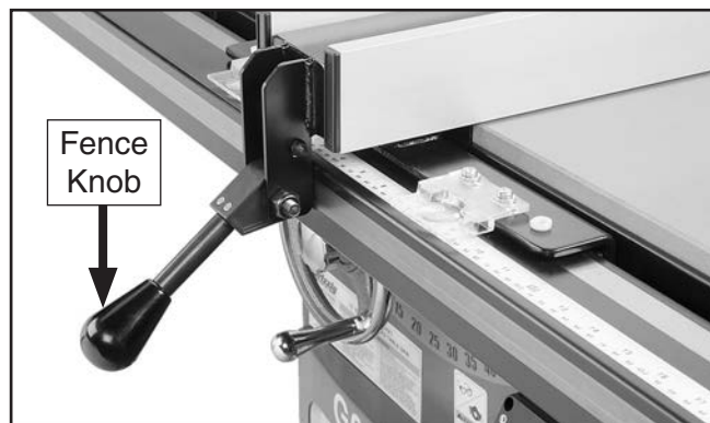
Figure 41. Fence knob installed.
