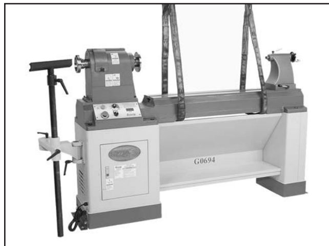
Figure 9. Lifting straps positioned to lift the lathe.
