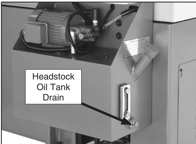
Figure 93. Headstock oil tank.
