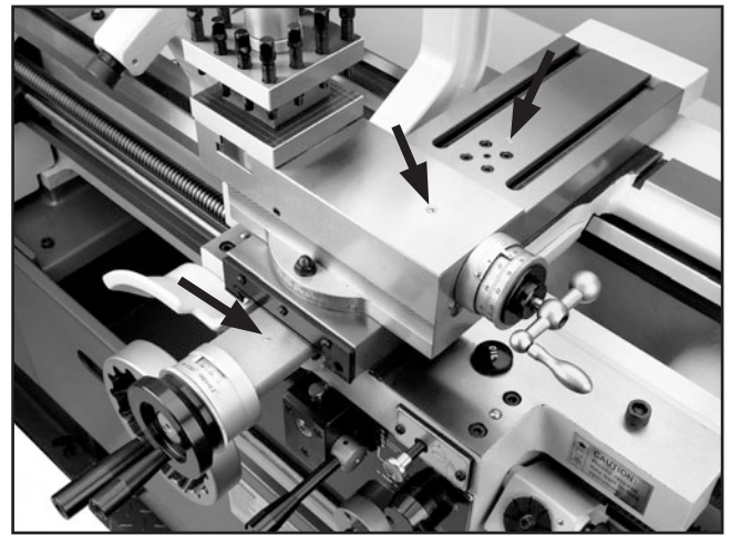
Figure 100. Ball oiler locations.
