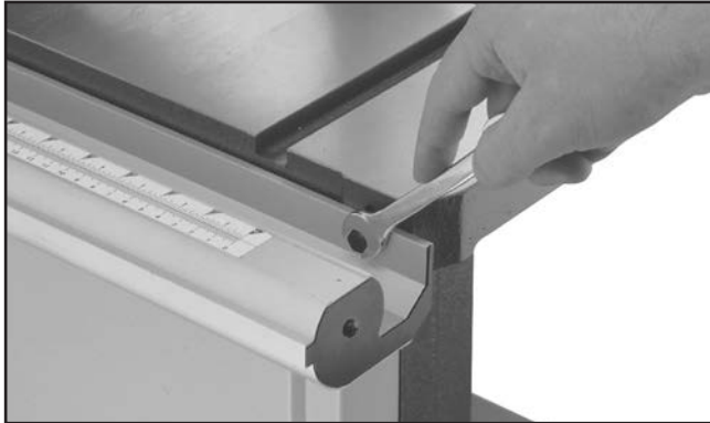
Figure 14. Fastening front fence rail to table.
