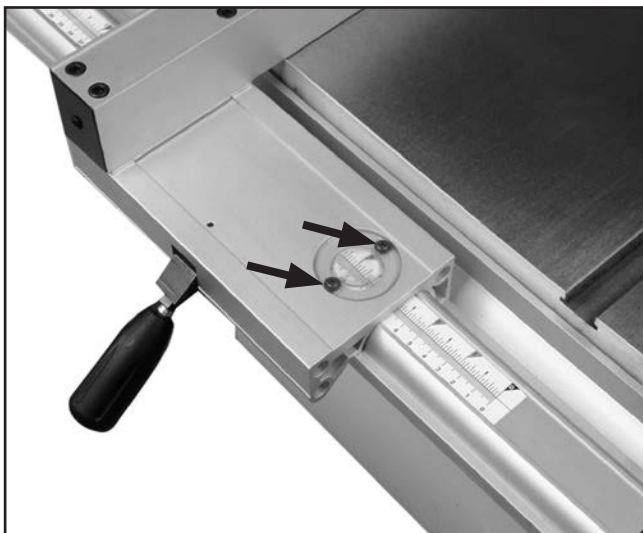
Figure 41. Scale recalibration screws.
