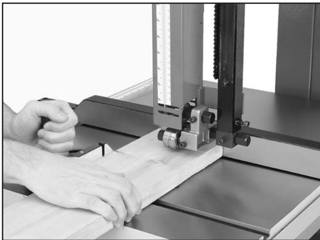
Figure 43. Typical crosscutting operation.
