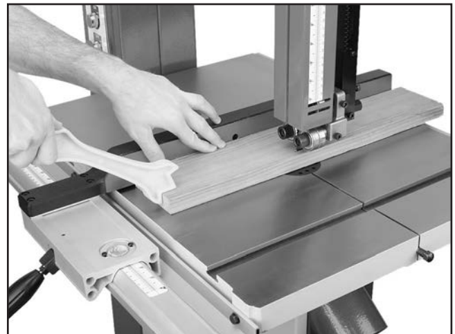
Figure 42. Typical ripping operation.
