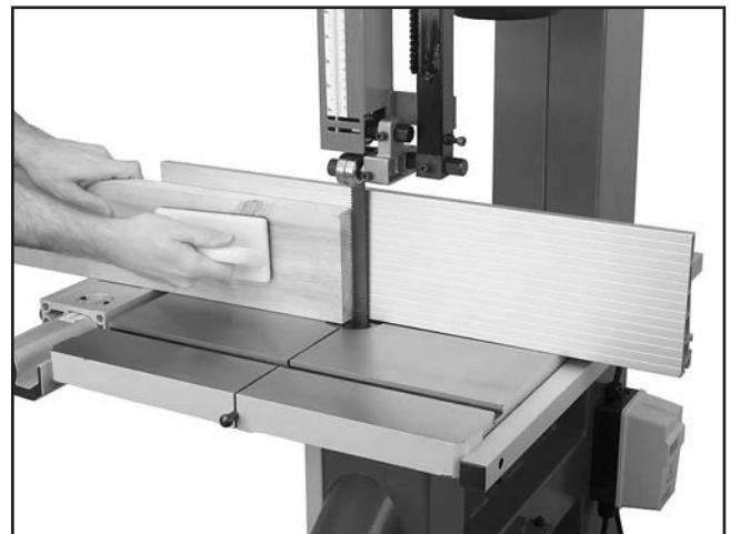
Figure 44. Typical resawing operation.
