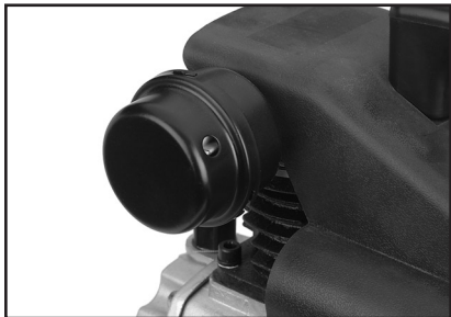
Figure 2. Air filter attached to cylinder head.
