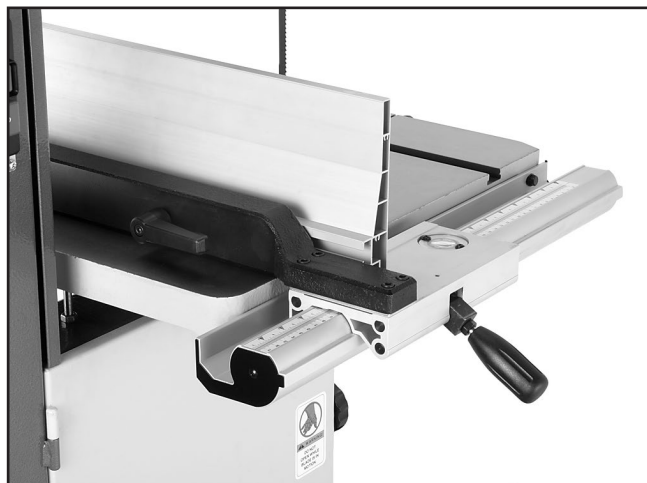
Figure 19. Correctly installed fence.
