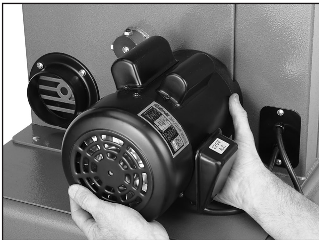
Figure 12. Installing motor (outside view).
