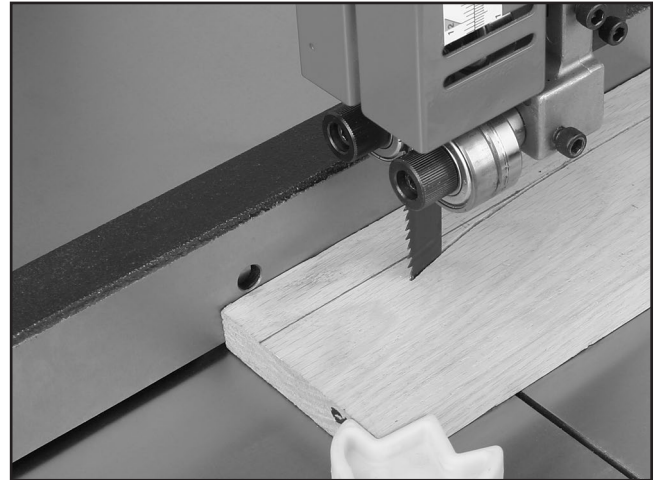
Figure 62. Blade leading away from line of cut.
