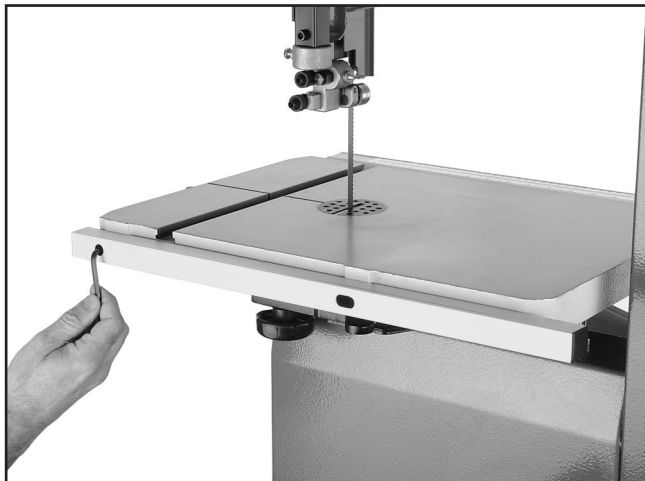
Figure 15. Rear rail installed.
