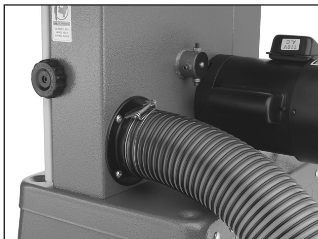
Figure 21. Dust hose attached to dust port.
