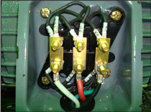
Figure 95. G0450 240V sanding drum motor wiring.
