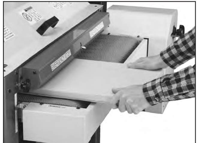
Figure 36. Example of using D3003 PRO-STIK® Cleaning Pad to clean sandpaper.
