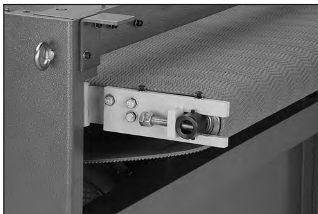
Figure 80. Conveyor belt loosened.
