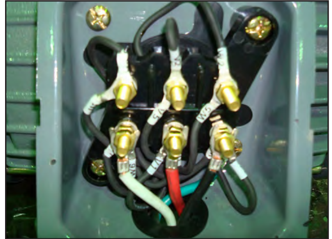
Figure 96. G0450 480V sanding drum motor wiring.
