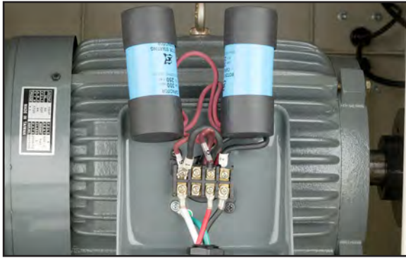
Figure 89. G0449 sanding drum motor wiring and start capacitors.
