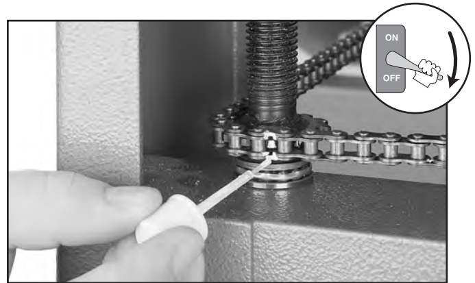
Figure 74. Marking sprocket tooth and chain.
