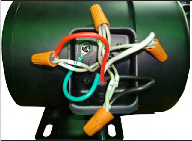
Figure 97. G0450 240V feed motor wiring.
