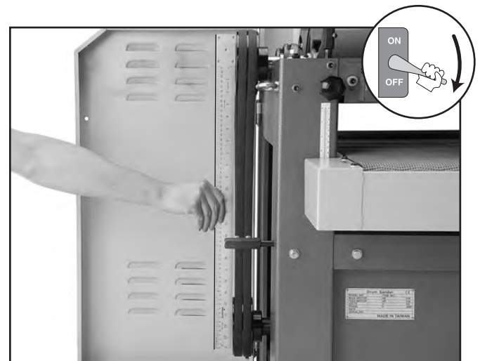
Figure 54. Checking pulley alignment with straightedge.
